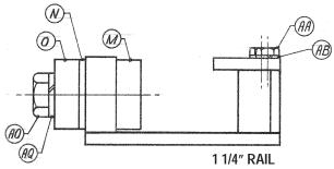
The roller assembly #11-300-25 is shipped loose. Insure that the L-rod (S) is threaded 1/2" into the fork (P). Align the L-rod (S) as shown and tighten nut (AI) against fork (P). Insert assembly into tension bracket (J) and install safety cover plate (T). See page 8, detail 2. Place safety retraction arm (K) over the L-rod (S) and fasten to side stile (A). See pages 4, 7 & 8.
